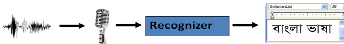
Figure 1.1 Overview of Speech Recognition System
